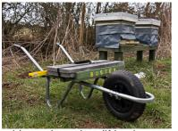
The precise construction details are dependent upon the wheelbarrow frame you've acquired. I built the platform from a single piece of 18mm thick exterior plywood, 52cm x 52cm. I braced this underneath using two pieces of 46mm x 21mm softwood. You should only fit a 'lip' at the front - to stop boxes sliding forward when it's in use - omit them from the sides and the back as this makes lifting boxes on and off easier and allows you to transport items wider than the
