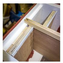
Construction is relatively simple, requiring little more than a sheet of 6mm ply, some offcuts from the scraps box, some softwood, a couple of G clamps, wood glue, screws and - inevitably - Elastoplast. I used the central divider as a sort of spine, to which I attached 15mm ply end panels, spaced the correct distance apart to fit a National frame. The easiest way to do this is to add some 8mm - beespace - softwood to the sidebars of a brood frame and then just mark where
